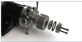
A quad seal is used on the end cap to reduce the loss of compressed air and lubrication during operation. It also provides a precise fit when assembled in the bush or directly into the section.
