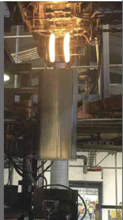
Lattimer engineers were tasked with re-engineering the units and adding in technical benefits and advancements where possible. The Lattimer units are manufactured from stainless steel keeping all waterways corrosion free, maximising the cooling effect and extending service life. All machining is carried out in-house and welding completed by a specialist coded welder.
